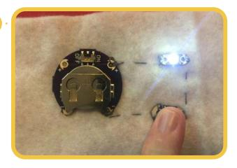
Test your circuit! Make sure the battery is in with the + sign facing up, make sure the switch on the battery holder is on, then press your button switch to turn on the LED light! If your circuit doesn't work, check closely for loose threads on both sides of the felt, and cut them short. Make sure the components are tightly attached with conductive thread.
