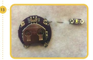
Make running stitches and join the positive +side of the LED to the felt. Tie off and cut the thread when you are done.
