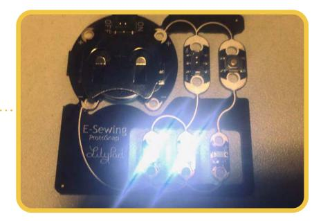
The components of the lilypad board can be broken apart to stitch into projects. We can join these components with any conductive material. Twist and break your lilypad components away from the board to separate them.
