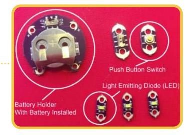
Try recreating the circuit below by joining the circled components with alligator clips. Pay attention to the orientation of the LEDs and battery. Be sure to connect the positive (+) side of the LED to the positive (+) of the battery. If they are connected backwards the circuit won't work. To test, make sure the switch on the battery is on, then turn the other switch in your circuit on!
