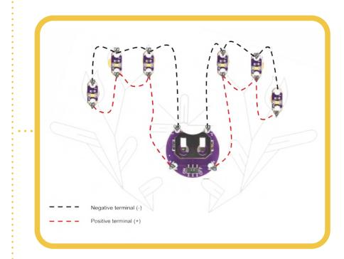
Here's a diagram identifying the orientation and placement of the LEDs and the battery holder. The broken lines indicate where the conductive thread will be sewn
