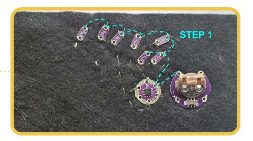
The final LED will connect to the negative terminal on the LilyTiny component.
