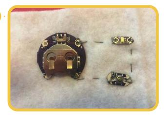
Make a knot and join the negative - side of the LED to the felt, with running stitches going to the button switch. Tie off again and cut. Tie a knot again on the other side of the switch, with running stitches going to the negative - of the battery. Tie off and cut the thread.
