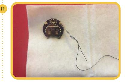
Attach the battery holder, stitch a knot and make several loops to secure.
