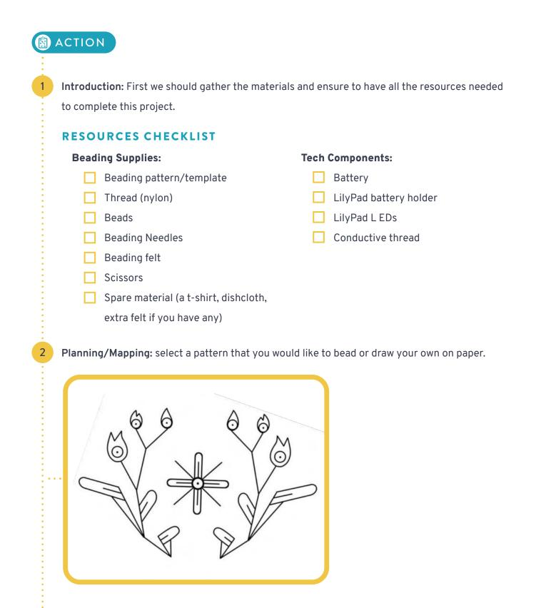
Identify parts you would like to highlight. Highlighted in yellow is where the LEDs will go on the template. This project requires six (6) LEDs in total.
