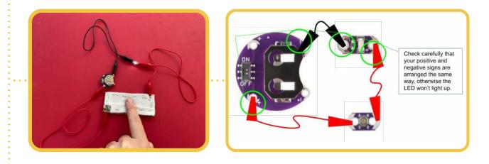
If you would like to use this switch in a wearable project, replace the alligator clips with conductive thread, and use regular thread to stitch the switch on to your project. You've now made a soft switch that can be used to control a light!
